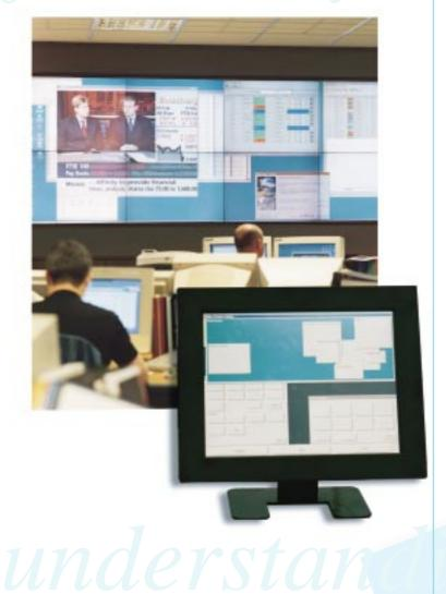
Controlling which applications are launched, when, and how they are positioned on the display wall gives operators easier, faster access to required information.
